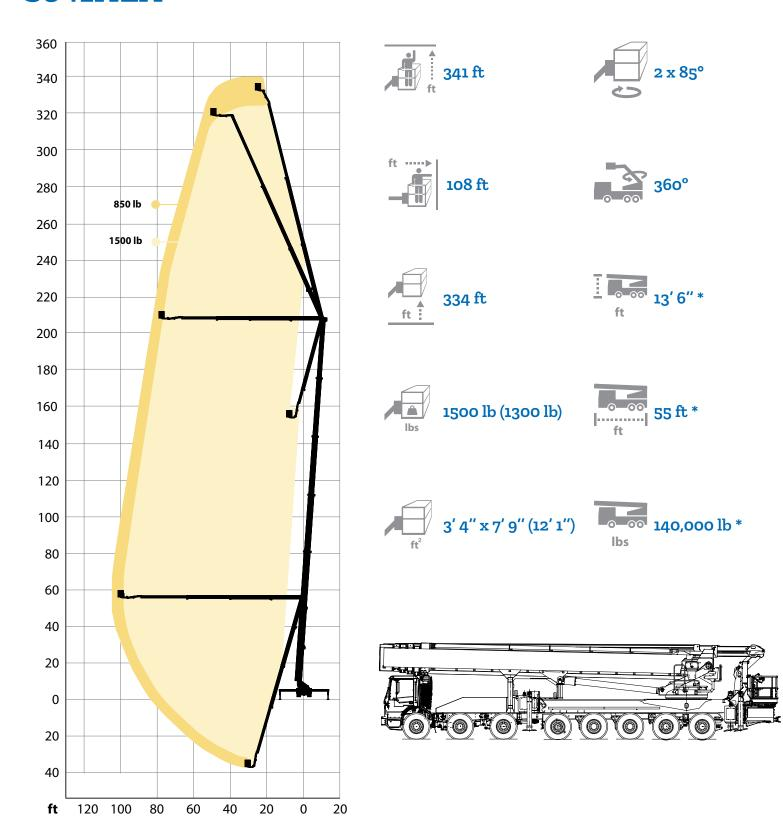
Diagrams presented with standard cage. Drawings with an example configuration and carrier, for reference purpose only. Variations apply. \*depending on the chassis
