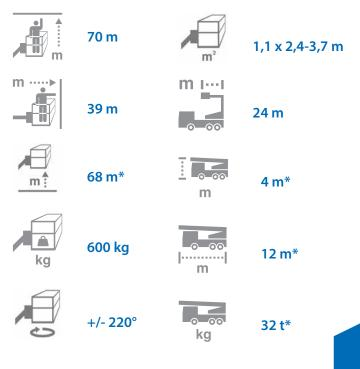
Diagrams presented with standard cage and standard cage rotation. Variations apply. \* depending on chassis
