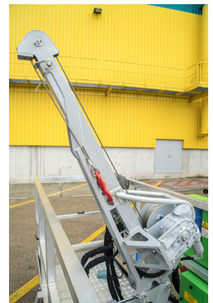
+/- 45 degrees slewing and extendable lifting jib.
