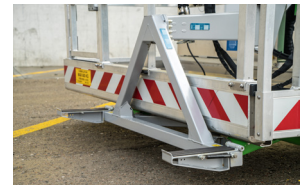
Standardised cage attachment points and fold-out feet for lifting.
